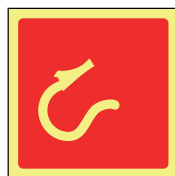
50347 Hose box with spray/jet fire nozzle
