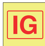
50356 Inert gas installation
